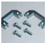
I. Mitsubishi Rear Shims Special spacers and longer fasteners shim the upper control arms for positive adjustment up to 1.5 degrees.
