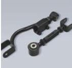
S. Adjustable Links Rear camber links adjust +/- 3.0 degrees without affecting wheel setback. Also includes upgraded rubber bushing material for improved handling. (S14)
