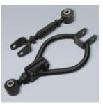
R. Adjustable Links Adjusts +/- 3.0 degrees of camber without affecting wheel setback. Also Includes upgraded stiffer rubber bushing material for improved handling. (S13)
