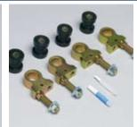
**C. Pivot Mounts** Steel replacement pivot mounts relocate the OEM upper control arms for positive camber adjustment up to +1.75 degrees. Includes polyurethane bushings and complete hardware.
