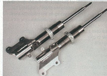
▲ In addition to their threaded outer bodies, coilover shocks are always a higher-cost, premium option, therefore they use premium valving and construction. In other words, they're good shocks. Also, these shocks are rebuildable by Progress Group, which is nice after several seasons of track action.
