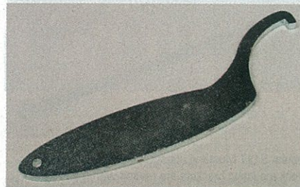
▲ While the adjusting collar can often be turned by hand, especially if the suspension is at full droop, a special wrench is supplied to rotate the collar in case it is tightly loaded.
