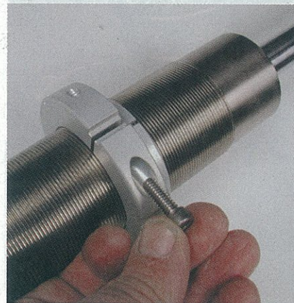
▲ Progress Group gives all its adjusting collars a lock bolt. Tightening the bolt pinches the collar, which is cut into a C-shape, holding it firmly to the strut body. To adjust the collar, the pinch bolt is loosened with an Allen wrench and the collar spun around.
