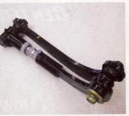
To get the alignment close, place the stock link and adjustable link side by side and adjust the turnbuckle assembly until they're the same length.
