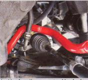
Looking from the passenger-side wheel well, be sure the anti-roll bar is located on the inboard side of this power steering hose. Positioning the bar on the outer side will ultimately kink the hose.
