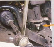
The nut in the center must be removed to drop the crossmember. To access it through the hole in the lower control arm, use a 19mm socket and an extension.
