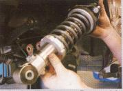
Before installing the rear coil-overs, rotate their upper mounting plates in proper orientation with their lower mounts. The upper mounting plates only attach to the car one way and can be difficult to turn once the coil-overs are compressed.
