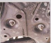
These are two of the four steering rack nuts. Their torque ratings are only 45 ft-lb, but they feel like much more. The base of the nuts feature anti-slip grooves that grab the metal and make them difficult to loosen.
