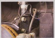
Unbolt the brake line bracket and unclip the ABS wire from the strut. The two bolts connecting the strut to the upper control arm must be removed, allowing the arm to drop. Note: Although front camber is nonadjustable, a slight amount of play may be found here by pulling or pushing on the upright before these two bolts are tightened.
