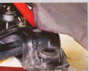
Notice the gap between the crossmember and the frame. If the crossmember is lowered this much, the stock anti-roll bar will have room to come out.
