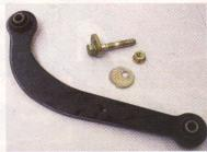
Rear camber adjustments are made on stock tCs using this camber bolt, which is retained even when using the adjustable camber links. Before tightening the cam bolt, make sure they're adjusted to their maximum outboard position.
