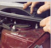
Two plastic clips on each side of the cowl must be removed in order to gain access to the strut's rearmost upper mounting nuts. Even with cowl pried out of the way, clearances are still tight and only a wrench will fit.
