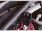
Installing coil-overs and the strut tower brace at the same time will save some labor. The Hotchkis Tuning strut brace brackets bolt directly to the front strut upper mounting plates, which need to be removed anyway when installing the coil-overs.
