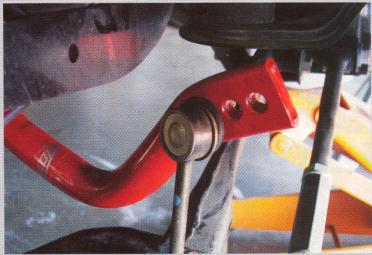
The Hotchkis anti-roll bars offer three-position adjustability. For maximum roll stiffness, bolt the end link to the innermost hole. Moving the end link outward decreases stiffness. The front bar can be set to a maximum of 68-percent stiffer than stock and the rear a maximum of 338 percent.
