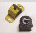
Since clearances are tight underneath the tC, it's best to wait to install the bushings and brackets until after the bar is finagled into place. Hotchkis provides grease for the bushings. Use it to avoid squeaks.
