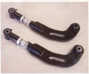
The Hotchkis Tuning rear camber links feature quiet, polygraphite bushings and a double-adjustable design. Once the jam nuts are loosened, camber may be adjusted by spinning the turnbuckle.
