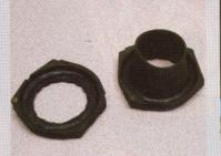
The original rear dust covers won't slide over the coil-overs unless they're trimmed. Cut them in half and use only the thin, ring-shaped portion.
