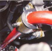
Grease fittings are integrated into the new anti-roll bar brackets to add additional lubricant. New hardware is also included.
