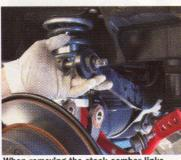
When removing the stock camber links, loosen the 17mm bolt connecting to the upper control arm first. It's easier to reach the inner bolt once the arm is swung upward.
