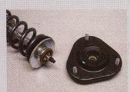
The stock upper mount must be reinstalled on the Progress coll-over. Everything else is included from Progress, including the nut that holds it in place.
