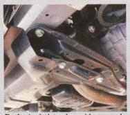
The front splashguards must be removed in order to access the bolts for the bridge bracket. A series of plastic screws and rivets must be popped out in order to remove the two pieces.
