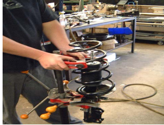
Using a spring compressor remove the spring from the strut
