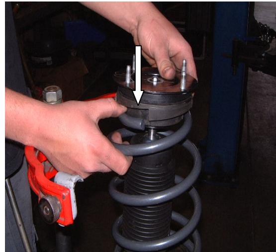
Align the upper spring mount with the spring keeping the alignment of the hat and vehicle in line. Torque all bolts to factory specifications.
