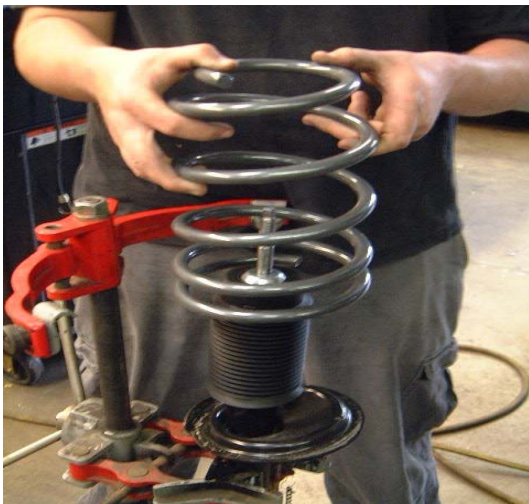
Place trimmed bump stop and dust boot back on the strut. Align spring on lower spring seat.
