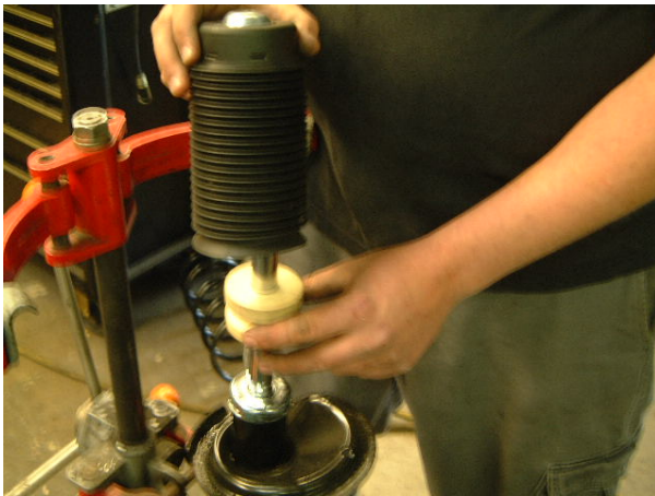
Remove dust boot and bump stop
