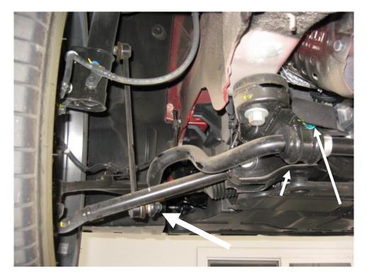
2. Remove end links from the bar end. Remove bushings and brackets. Remove stock bar.
