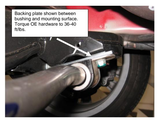
3. Apply grease to the inside of the new bushings. Use the backing plate between the chassis and the new bushing as shown. Attach your new Progress bar in the same position as the stock bar using factory hardware.
