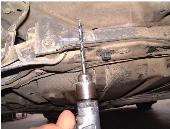
Figure 4: Drill through the rear lip of the cross member
