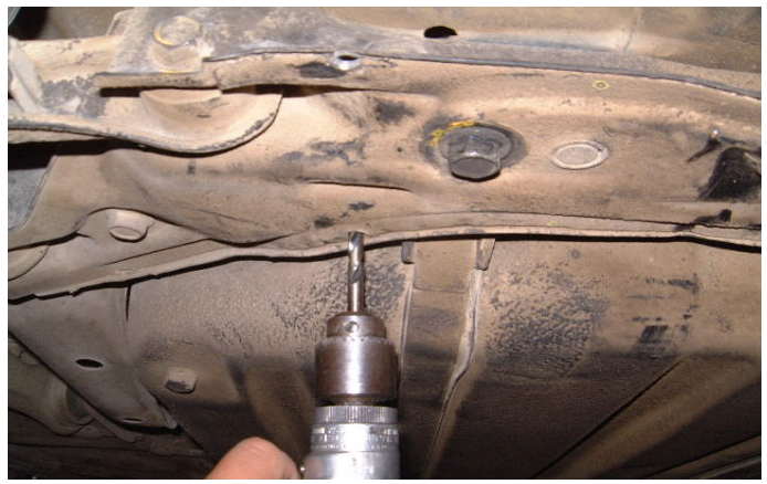
Figure 5: Drill through the front lip of the cross member
