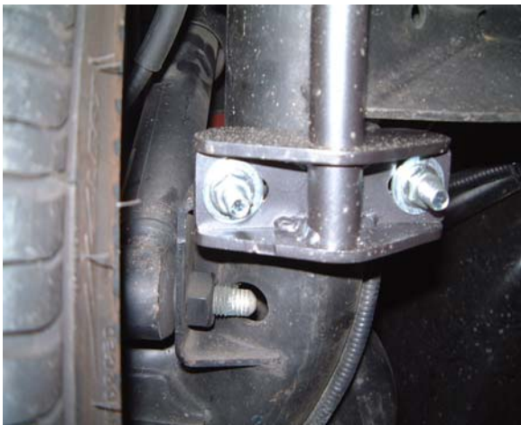
Saddle shown over the lower shock bracket Driver side
