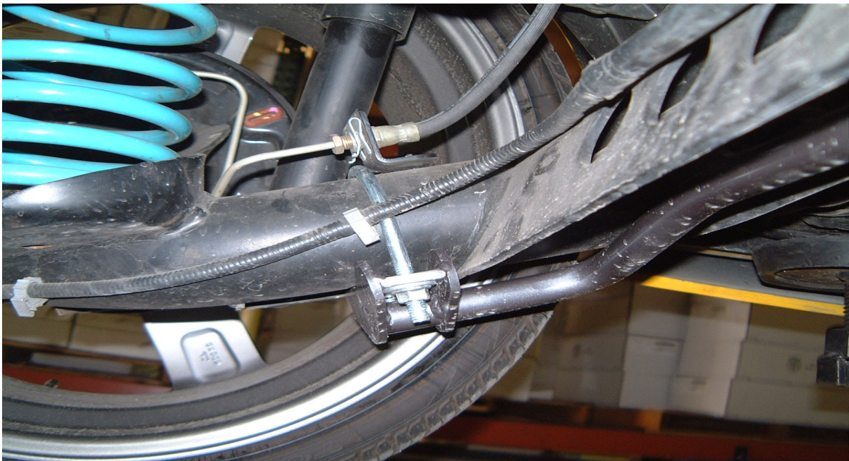
Driver side U-bolt placement behind the brake line bracket
