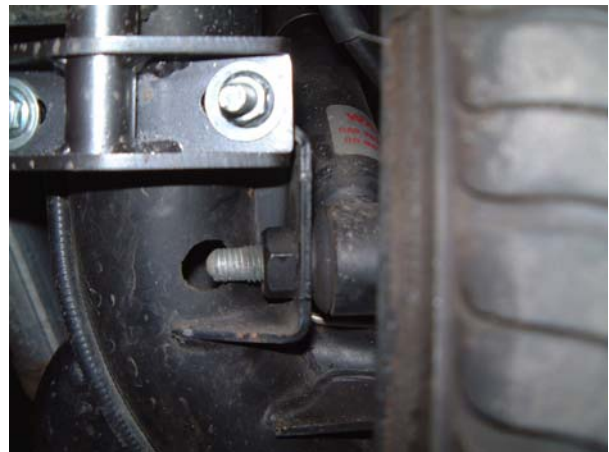
Saddle shown over the lower shock bracket Passenger side
