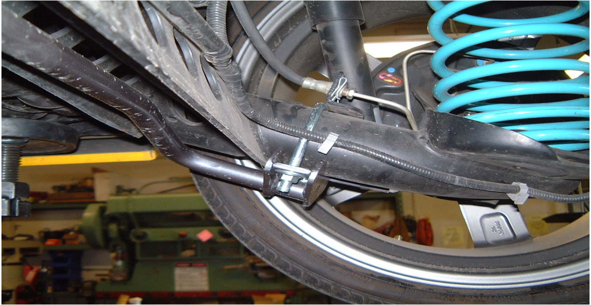
Passenger side U-bolt placement in front of the brake line bracket
