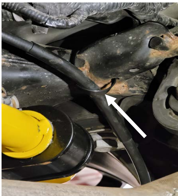
Use zip tie to secure e-brake cable. (Figure E)
