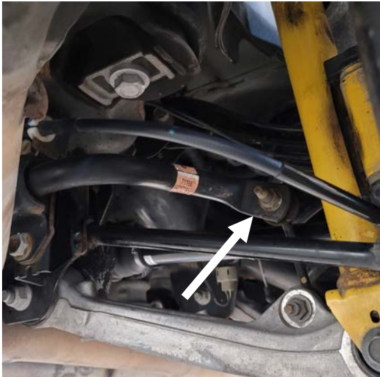
Remove the nuts that attach sway bar to end link. (Figure A)
