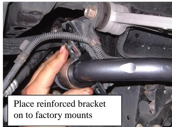
Place reinforced bracket on to factory mounts
