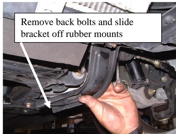
Remove back bolts and slide bracket off rubber mounts
