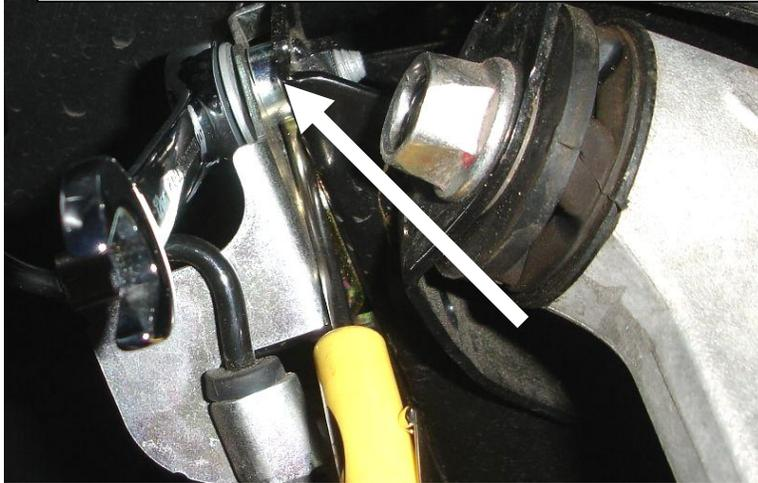
3. Attach end link, radiator mounts and ABS wires **with spacer behind it**. Torque all fasteners to factory specifications. Attach splash tray then install wheels and tires. Lower the front of car onto ground, and roll car back and forth to settle suspension.
