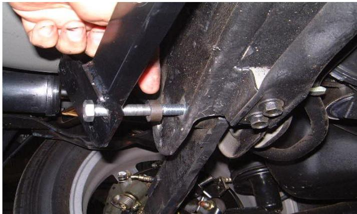
Figure A M12 bolt, washer and spacer tube in position.
