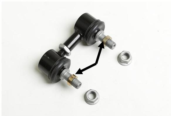
We have included four end link spacers. If your vehicle is not lower than 1.5" (38mm) your installation will NOT require any spacers. These spacers are provided to adjust the end link angle for best function and durability.
