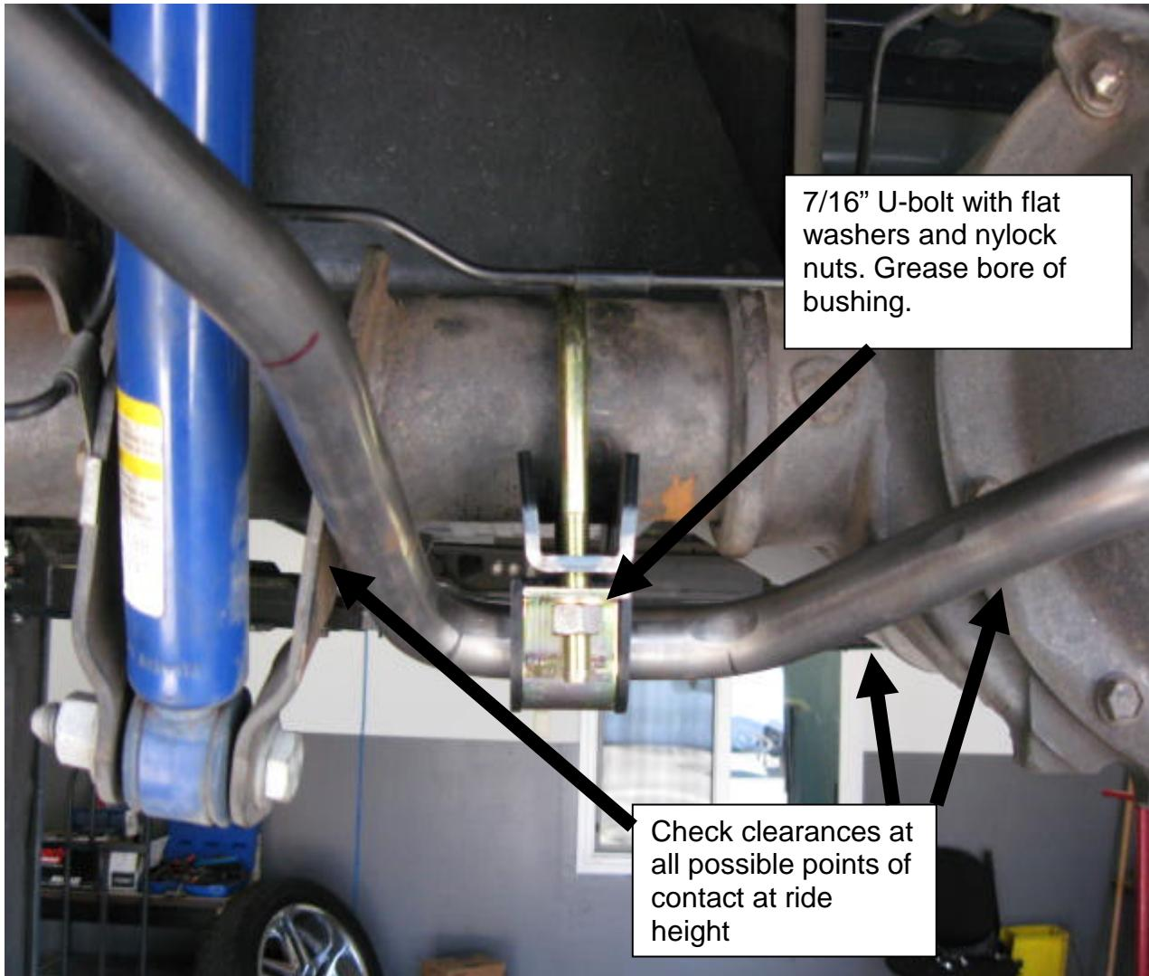
3. Grease the bore (inside) of the supplied bushing. Open the bushing and place it over the bar then place the bracket over the bushing. Align the u-bolt over the axle and through the saddle and bracket. Hand tighten both bushing bracket mounts.
