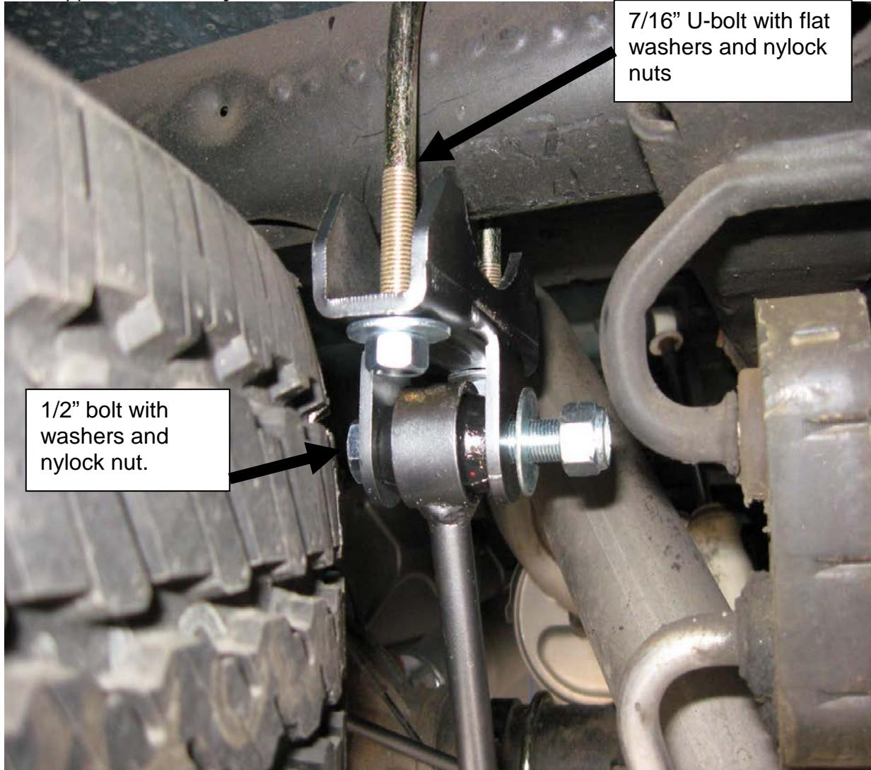
2. Loosely assemble the upper saddles on the cross member in front of the spare tire as shown. Make sure to move any electrical wires that may interfere with the mounting location (both sides of the spare) on the cross member. Attach end link as shown with the head of the bolts towards the center of the truck. Do not tighten at this time.
