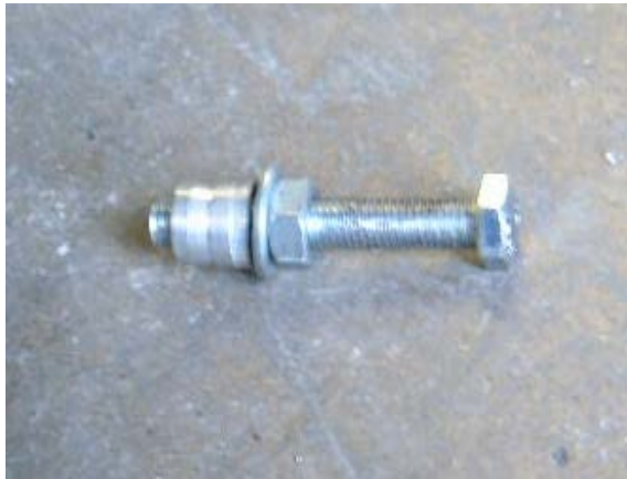
Figure 1 Nutsert shown ready to install
