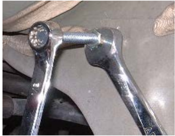
Figure 2 Hold bolt head and turn nut until tight
