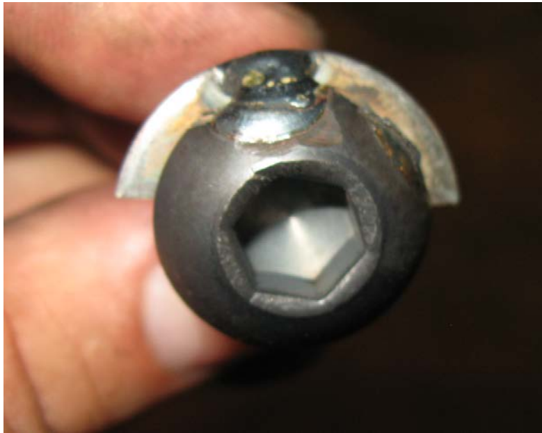
M12-1.75 x30 Button Head with half washer. Half washer should fully seat in step on spring perch.
